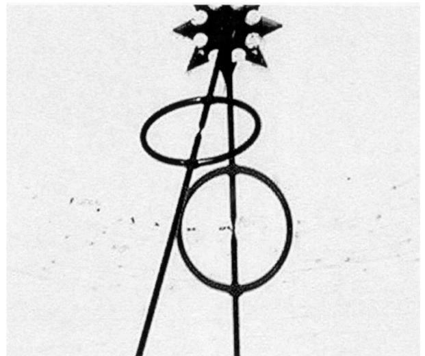
**Fig. 4.** Close-up of the nodus (upper circle) and its shadow (lower circle) on the winter solstice. The dark pencil marks are from observations recorded at earlier times that solstice morning. The lighter marks connected by faint lines of declination were recorded on previous days that autumn.
